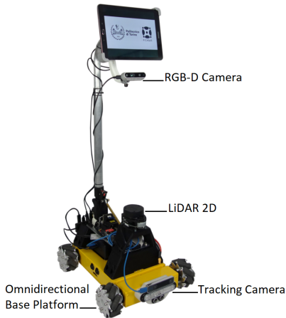
Fig. 2: The omnidirectional platform we set up for experimentation and validation of our novel methodology.
