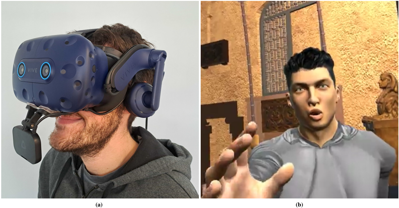
FIGURE 1 VR setup used for the experiment (HTC Vive Pro Eye + Facial Tracker) (a). Close-up of the user's avatar (b).
