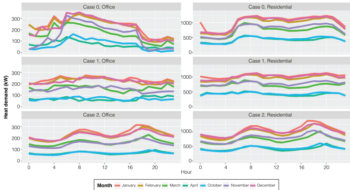
Figure 3: Average monthly heat loads for the offices and the residential buildings
