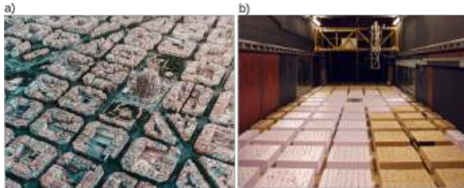
Figure 1: (a) Aerial view of the city of Barcelona (Spain). Source: Barcelona From Above by Ian Harper. (b) The modelled urban canopy in the wind tunnel.
