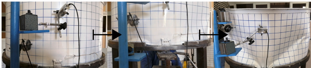
Fig. 4. Progressive buckling of a thin-walled steel tank subjected to local support settlement. Photos by courtesy of H. Naseri (Urmia University).
