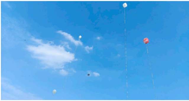
Fig. 12. Experiment with five tethered radiosondes at INRIM on September 29, 2021. Two radiosondes tracked using video camera were marked in red and black.
