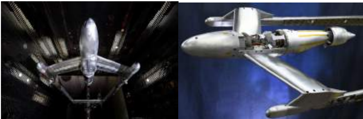
Figure 3: SUBLIME BLI360 configuration in wind tunnel
