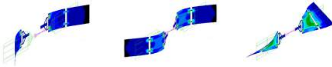
Fig. 2: Modal Strain Energy (MSE) map. From left to right, 1 st mode, 2 nd mode, 3 rd mode
