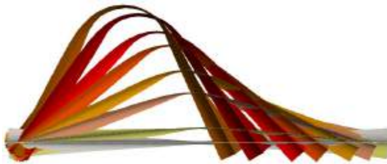
Figure 10 - Folding simulation of the TRAC longeron including contact mechanics
