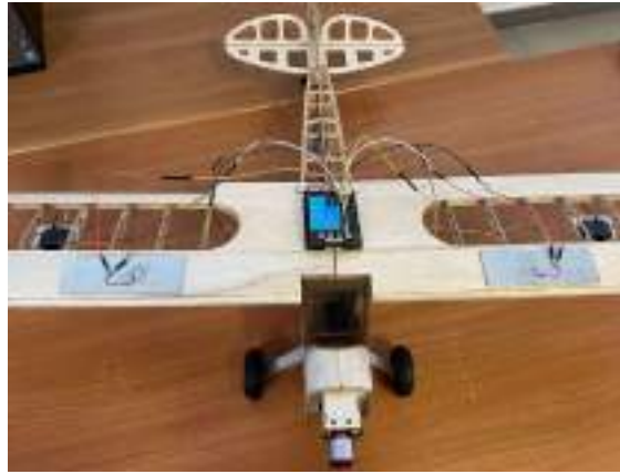
Fig. 1. Experimental setup: acquisition of the vibrations via Raspberry Pi
