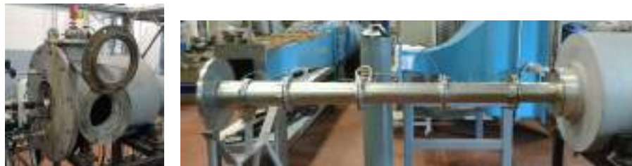
Figure 6 – VOF Test Chamber (left) and Diffuser (right).
