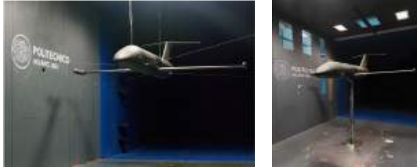
Figure 4: The XDIA model in free-free condition (left) and installed on the pylon (right)
