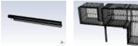
Fig. 2: Computational domain used in calculations
