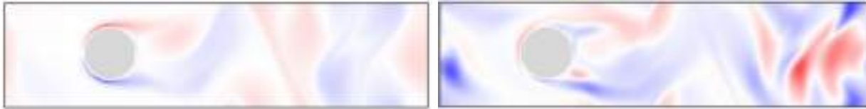
Figure 4 –Classical vs. quantum LBM algorithms results (vorticity)
