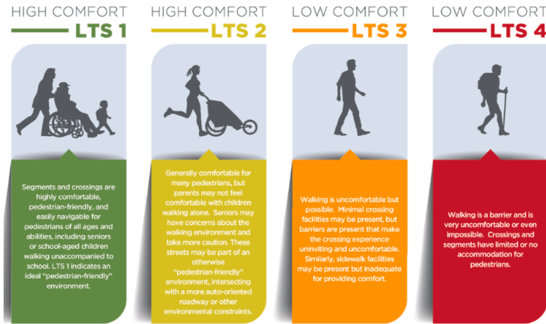
Fig. 3. Level of Traffic stress for pedestrians. Source: City of Boulder, 2019 Low-Stress Walk and Bike Network Plan .
