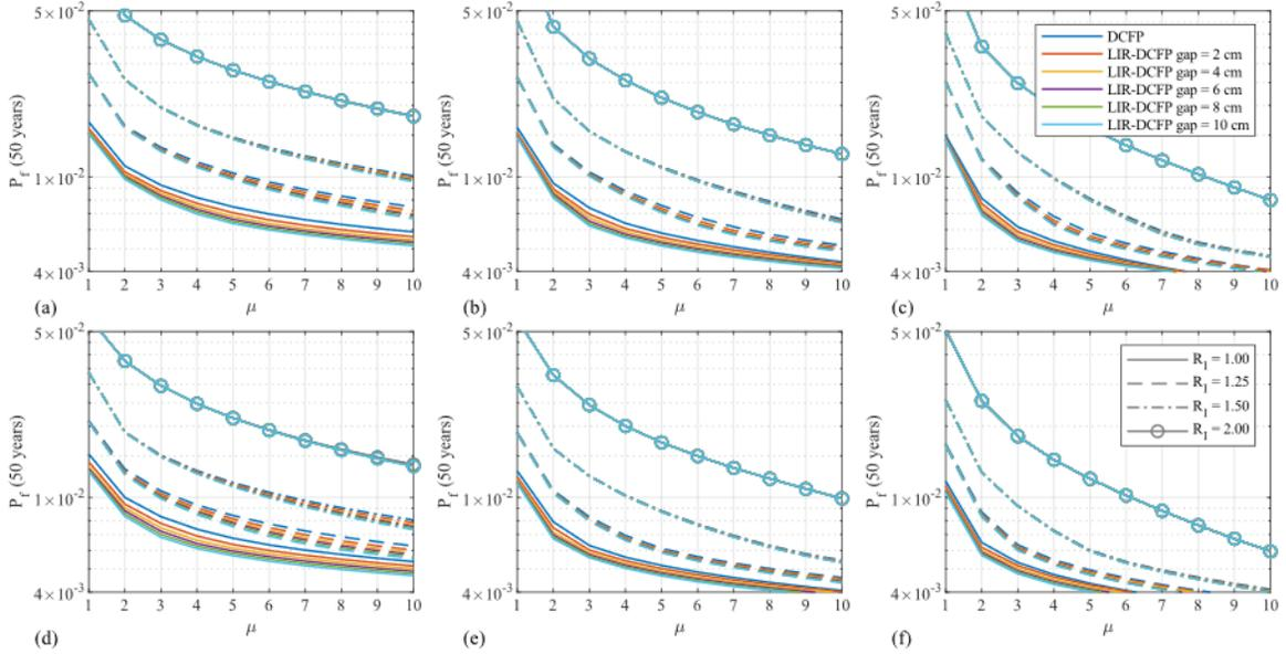
Figure 16: Seismic reliability of the superstructure for  $T_b = 3$  sec and  $r_H = 0.05$ : (a)  $\gamma = 0.7$  and  $T_s = 0.3$  sec; (b)  $\gamma = 0.7$  and  $T_s = 0.6$  sec; (c)  $\gamma = 0.7$  and  $T_s = 0.9$  sec; (d)  $\gamma = 0.9$  and  $T_s = 0.3$  sec; (e)  $\gamma = 0.9$  and  $T_s = 0.6$  sec; (f)  $\gamma = 0.9$  and  $T_s = 0.9$  sec.
