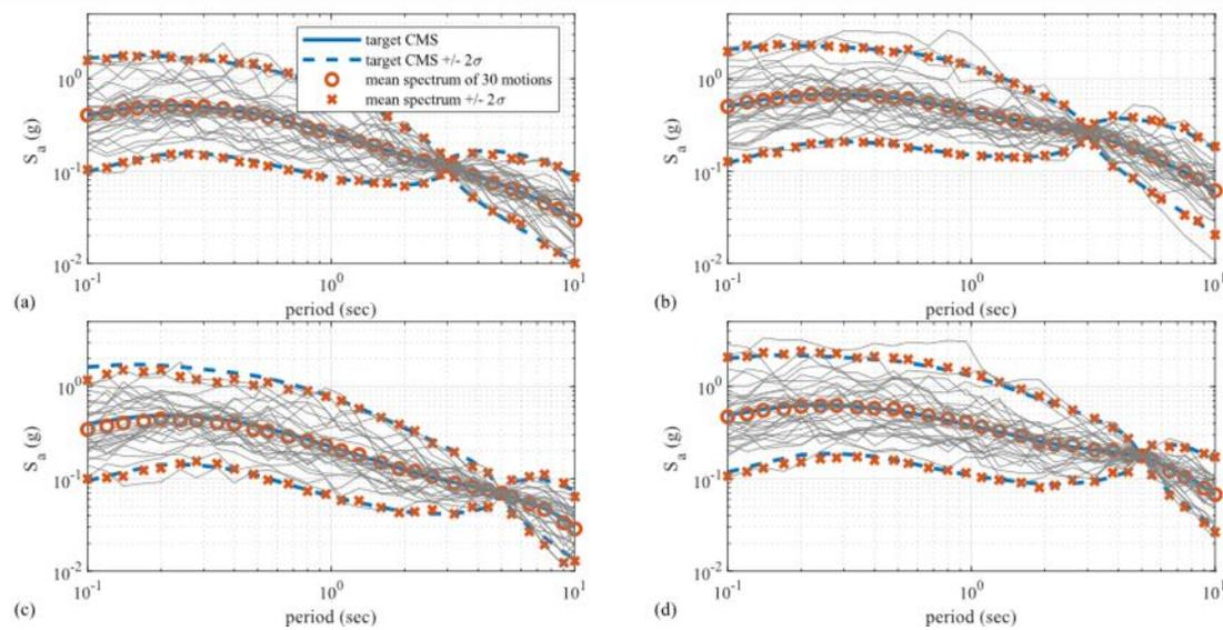
Figure 7: Spectra of the scaled selected ground motions for different  $T_r$  and conditioning periods  $T^*$ : (a)  $T_r = 475$  years and  $T^* = 3$  sec; (b)  $T_r = 2,475$  years and  $T^* = 3$  sec; (c)  $T_r = 475$  years and  $T^* = 5$  sec; (d)  $T_r = 2,475$  years and  $T^* = 5$  sec.
