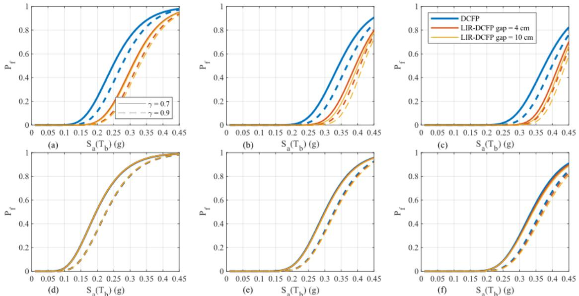
Figure 12: Seismic fragility curves of superstructure related to  $T_s = 0.3$  sec and  $r_H = 0.05$ : (a)  $LS_\mu = 1$  and  $R_I = 1$ ; (b)  $LS_\mu = 4$  and  $R_I = 1$ ; (c)  $LS_\mu = 7$  and  $R_I = 1$ ; (d)  $LS_\mu = 1$  and  $R_I = 2$ ; (e)  $LS_\mu = 4$  and  $R_I = 2$ ; (f)  $LS_\mu = 7$  and  $R_I = 2$ .
