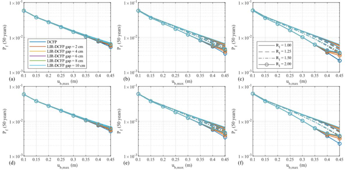
Figure 14: Seismic reliability of the isolation level for  $T_b = 3$  sec and  $r_H = 0.10$ : (a)  $\gamma = 0.7$  and  $T_s = 0.3$  sec; (b)  $\gamma = 0.7$  and  $T_s = 0.6$  sec; (c)  $\gamma = 0.7$  and  $T_s = 0.9$  sec; (d)  $\gamma = 0.9$  and  $T_s = 0.3$  sec; (e)  $\gamma = 0.9$  and  $T_s = 0.6$  sec; (f)  $\gamma = 0.9$  and  $T_s = 0.9$  sec.
