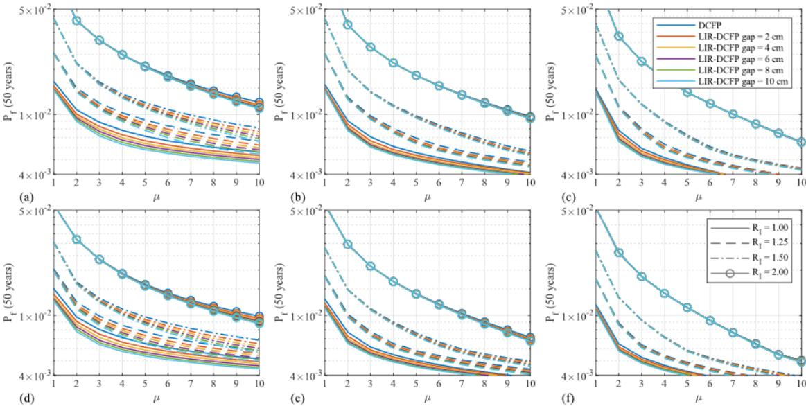
Figure 17: Seismic reliability of the superstructure for  $T_b = 3$  sec and  $r_H = 0.10$ : (a)  $\gamma = 0.7$  and  $T_s = 0.3$  sec; (b)  $\gamma = 0.7$  and  $T_s = 0.6$  sec; (c)  $\gamma = 0.7$  and  $T_s = 0.9$  sec; (d)  $\gamma = 0.9$  and  $T_s = 0.3$  sec; (e)  $\gamma = 0.9$  and  $T_s = 0.6$  sec; (f)  $\gamma = 0.9$  and  $T_s = 0.9$  sec.
