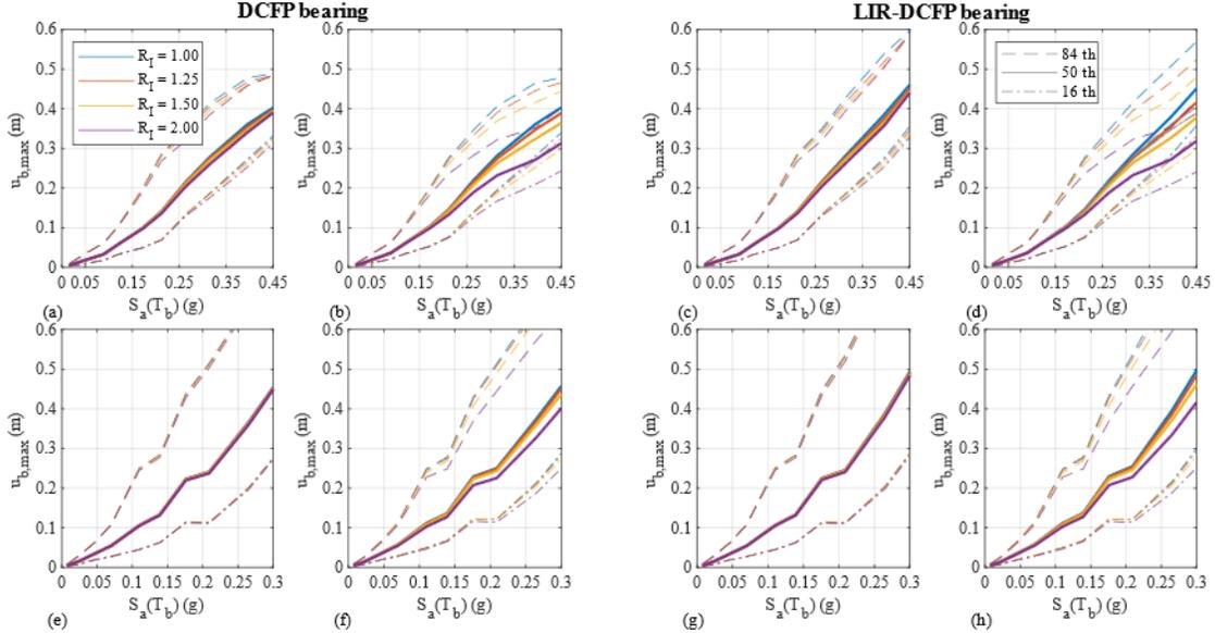
Figure 8: Incremental dynamic analyses curves of the isolation level with  $\gamma = 0.7$  and  $r_H = 0.05$ : (a) DCFP,  $T_b = 3$  sec,  $T_s = 0.3$  sec; (b) DCFP,  $T_b = 3$  sec,  $T_s = 0.9$  sec; (c) LIR-DCFP,  $T_b = 3$  sec,  $T_s = 0.3$  sec; (d) LIR-DCFP,  $T_b = 3$  sec,  $T_s = 0.9$  sec; (e) DCFP,  $T_b = 5$  sec,  $T_s = 0.3$  sec; (f) DCFP,  $T_b = 5$  sec,  $T_s = 0.9$  sec; (g) LIR-DCFP,  $T_b = 5$  sec,  $T_s = 0.3$  sec; (h) LIR-DCFP,  $T_b = 5$  sec,  $T_s = 0.9$  sec.
