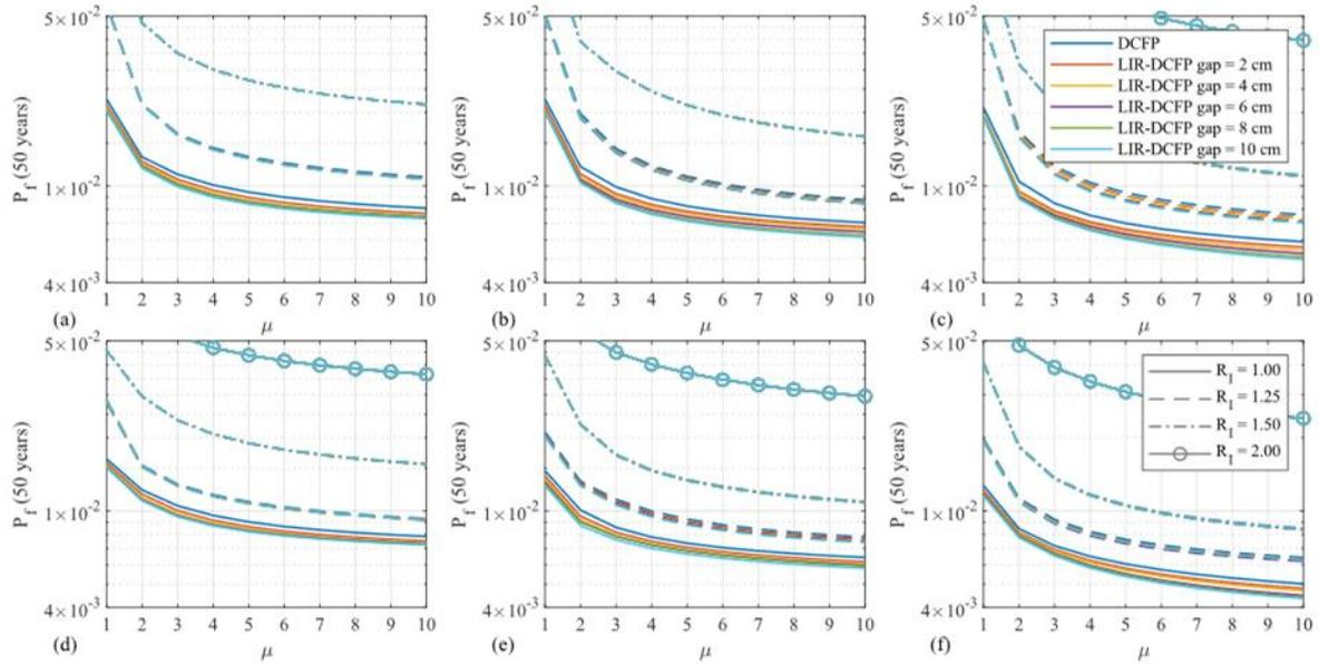
Figure 22: Seismic reliability of the superstructure for  $T_b = 5$  sec and  $r_s = -0.05$ : (a)  $\gamma = 0.7$  and  $T_s = 0.3$  sec; (b)  $\gamma = 0.7$  and  $T_s = 0.6$  sec; (c)  $\gamma = 0.7$  and  $T_s = 0.9$  sec; (d)  $\gamma = 0.9$  and  $T_s = 0.3$  sec; (e)  $\gamma = 0.9$  and  $T_s = 0.6$  sec; (f)  $\gamma = 0.9$  and  $T_s = 0.9$  sec.
