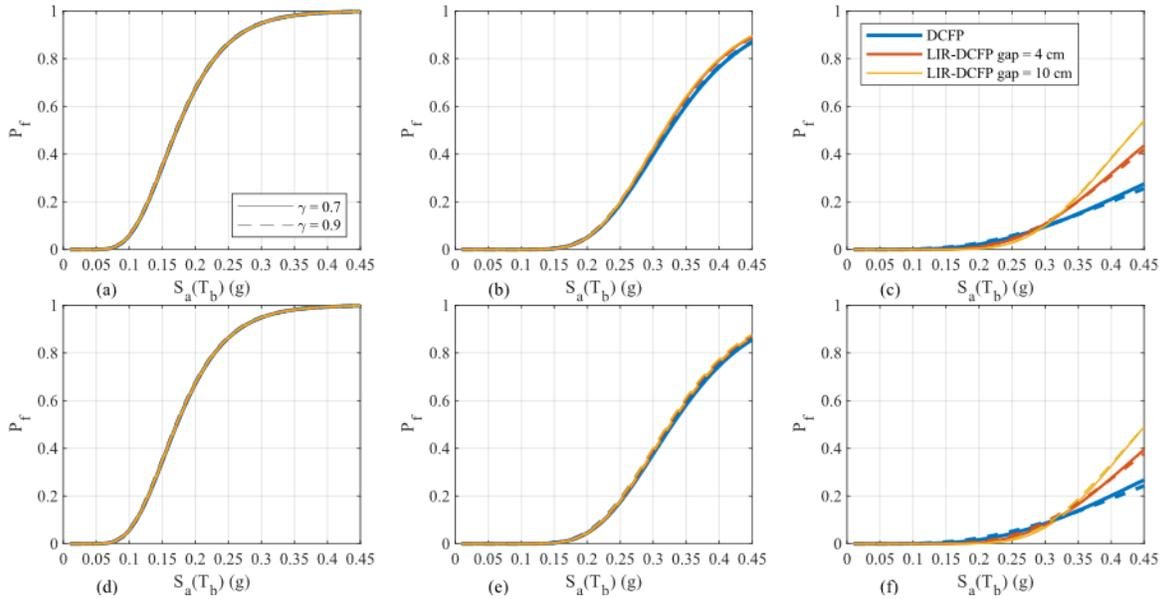
Figure 10: Seismic fragility curves of the isolation level related to  $T_s = 0.3$  sec and  $r_H = 0.05$ : (a)  $LS_{u_{b,max}} = 10$  cm and  $R_I = 1$ ; (b)  $LS_{u_{b,max}} = 30$  cm and  $R_I = 1$ ; (c)  $LS_{u_{b,max}} = 45$  cm and  $R_I = 1$ ; (d)  $LS_{u_{b,max}} = 10$  cm and  $R_I = 2$ ; (e)  $LS_{u_{b,max}} = 30$  cm and  $R_I = 2$ ; (f)  $LS_{u_{b,max}} = 45$  cm and  $R_I = 2$ .
