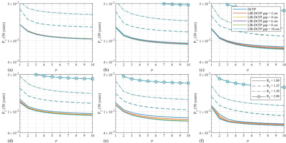
Figure 19: Seismic reliability of the superstructure for  $T_b = 3$  sec and  $r_s = -0.10$ : (a)  $\gamma = 0.7$  and  $T_s = 0.3$  sec; (b)  $\gamma = 0.7$  and  $T_s = 0.6$  sec; (c)  $\gamma = 0.7$  and  $T_s = 0.9$  sec; (d)  $\gamma = 0.9$  and  $T_s = 0.3$  sec; (e)  $\gamma = 0.9$  and  $T_s = 0.6$  sec; (f)  $\gamma = 0.9$  and  $T_s = 0.9$  sec.
