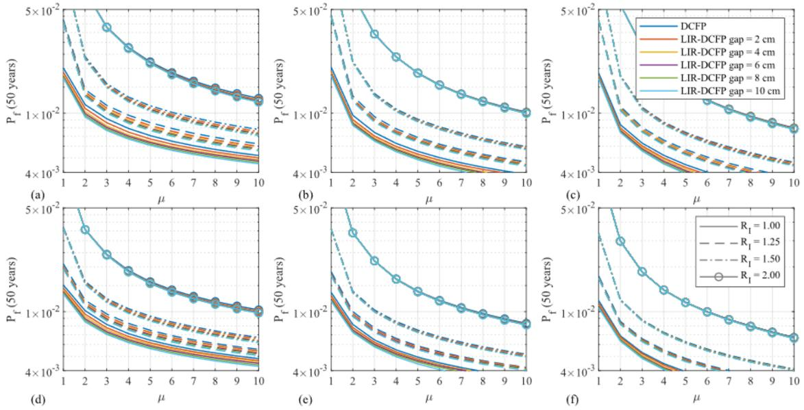
Figure 20: Seismic reliability of the superstructure for  $T_b = 5$  sec and  $r_H = 0.05$ : (a)  $\gamma = 0.7$  and  $T_s = 0.3$  sec; (b)  $\gamma = 0.7$  and  $T_s = 0.6$  sec; (c)  $\gamma = 0.7$  and  $T_s = 0.9$  sec; (d)  $\gamma = 0.9$  and  $T_s = 0.3$  sec; (e)  $\gamma = 0.9$  and  $T_s = 0.6$  sec; (f)  $\gamma = 0.9$  and  $T_s = 0.9$  sec.
