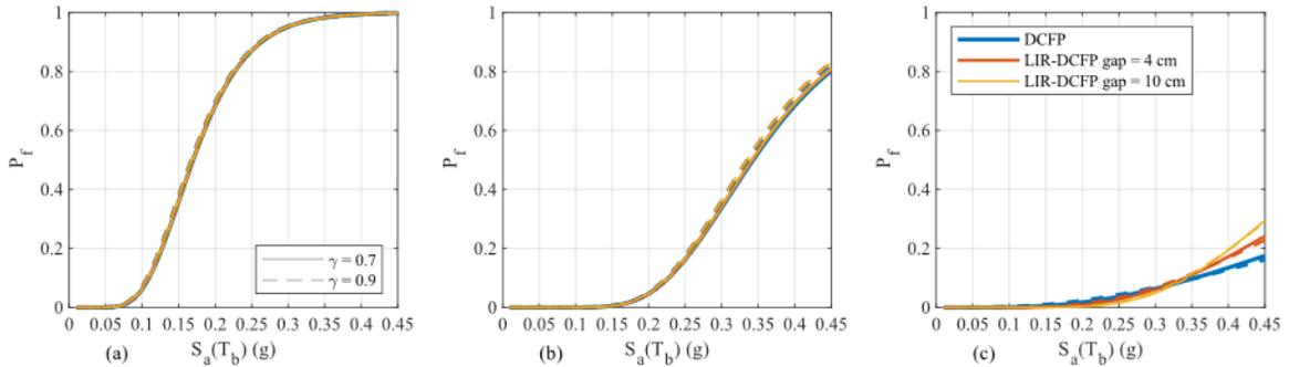
Figure 11: Seismic fragility curves of the isolation level related to  $T_s = 0.6$  sec,  $r_H = 0.05$  and  $R_I = 2$ : (a)  $LS_{u_{b,max}} = 10$  cm; (b)  $LS_{u_{b,max}} = 30$  cm; (c)  $LS_{u_{b,max}} = 45$  cm.
