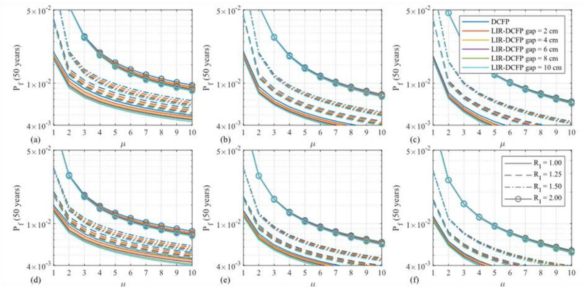
Figure 21: Seismic reliability of the superstructure for  $T_b = 5$  sec and  $r_H = 0.10$ : (a)  $\gamma = 0.7$  and  $T_s = 0.3$  sec; (b)  $\gamma = 0.7$  and  $T_s = 0.6$  sec; (c)  $\gamma = 0.7$  and  $T_s = 0.9$  sec; (d)  $\gamma = 0.9$  and  $T_s = 0.3$  sec; (e)  $\gamma = 0.9$  and  $T_s = 0.6$  sec; (f)  $\gamma = 0.9$  and  $T_s = 0.9$  sec.
