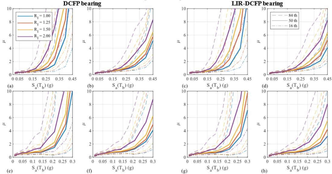
Figure 9: Incremental dynamic analyses curves of the superstructure with  $\gamma = 0.7$  and  $r_H = 0.05$ : (a) DCFP,  $T_b = 3$  sec,  $T_s = 0.3$  sec; (b) DCFP,  $T_b = 3$  sec,  $T_s = 0.9$  sec; (c) LIR-DCFP,  $T_b = 3$  sec,  $T_s = 0.3$  sec; (d) LIR-DCFP,  $T_b = 3$  sec,  $T_s = 0.9$  sec; (e) DCFP,  $T_b = 5$  sec,  $T_s = 0.3$  sec; (f) DCFP,  $T_b = 5$  sec,  $T_s = 0.9$  sec; (g) LIR-DCFP,  $T_b = 5$  sec,  $T_s = 0.3$  sec; (h) LIR-DCFP,  $T_b = 5$  sec,  $T_s = 0.9$  sec.
