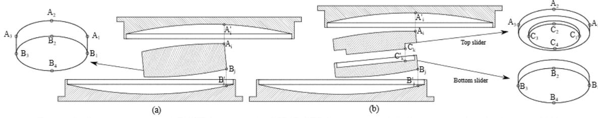
Figure 2: Contact points: (a) DCFP bearing; (b) LIR-DCFP bearing (modified from Auad and Almazán [21]).
