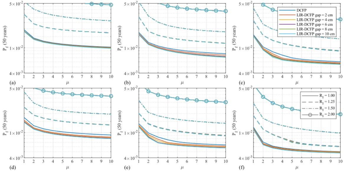
Figure 18: Seismic reliability of the superstructure for  $T_b = 3$  sec and  $r_s = -0.05$ : (a)  $\gamma = 0.7$  and  $T_s = 0.3$  sec; (b)  $\gamma = 0.7$  and  $T_s = 0.6$  sec; (c)  $\gamma = 0.7$  and  $T_s = 0.9$  sec; (d)  $\gamma = 0.9$  and  $T_s = 0.3$  sec; (e)  $\gamma = 0.9$  and  $T_s = 0.6$  sec; (f)  $\gamma = 0.9$  and  $T_s = 0.9$  sec.
