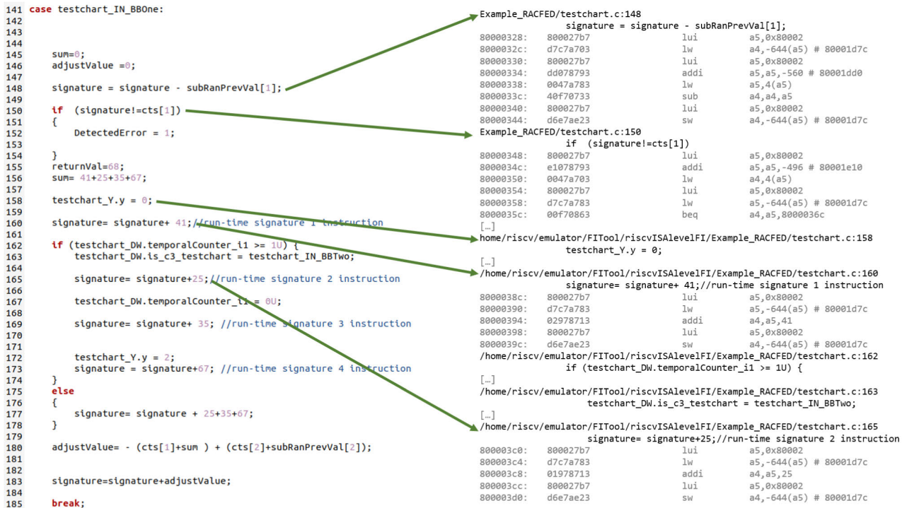
FIGURE 3. Mapping between the signature updates instructions in C and the relative Assembly (RISC-V RV32I) translation. It is possible to see that GCC, configured with O0 optimization settings, keeps the instructions in order.
