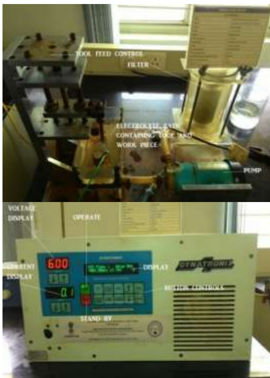
Fig. 1: Micro ECMM setup and pulse rectifier
