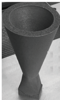
Fig. 1. Prototype of the Ka-band feed in AlSi10Mg alloy still attached at the building platform. In the bottom part it can be observed the presence of supports for the WR28 flanges.
