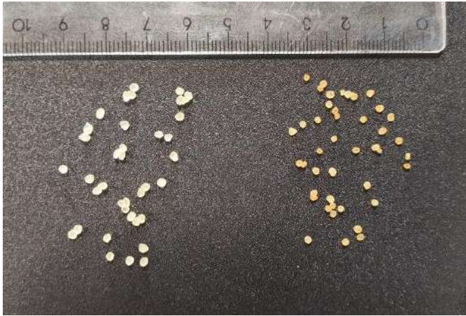
Figure s1: Beads of CaAlg ‘as produced’ (left) and ‘after 40 cycles’ (right).
