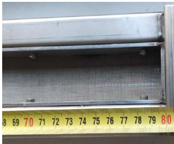
Figure s19: Detail of the fine mesh used to cover the exchanger sides, keeping the material inside. A ruler (in cm) is placed for reference.
