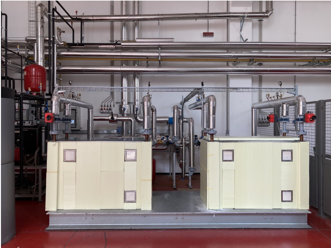
Fig. 3.14 "TopOpt" (left) and "Longitudinal" (right) LHTS units in the laboratory environment
