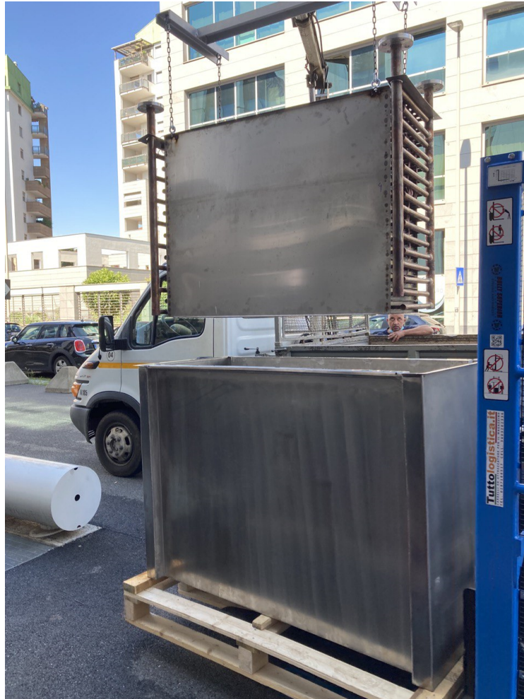
Fig. 3.7 Assembly of LHTS inner heat exchanger and external case
