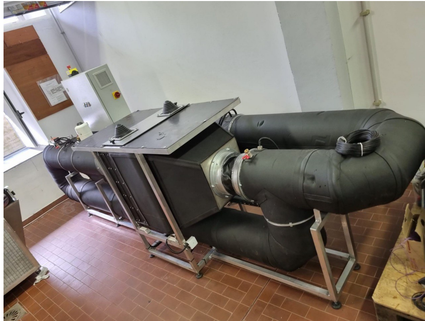
Fig. 6.9 Detail of the Hybrid Solar Cooling prototype
