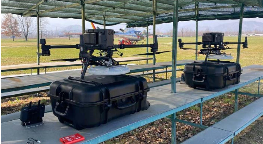
Figure 2: UAVs equipped with antenna, Raspberry Pi, and power bank.
