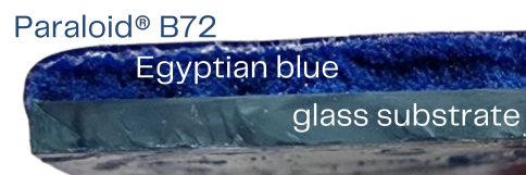
Fig. 8.2 Example of the stratification obtained in the samples from the second sets with Paraloid ® B72 deposited on a background layer of Egyptian blue
