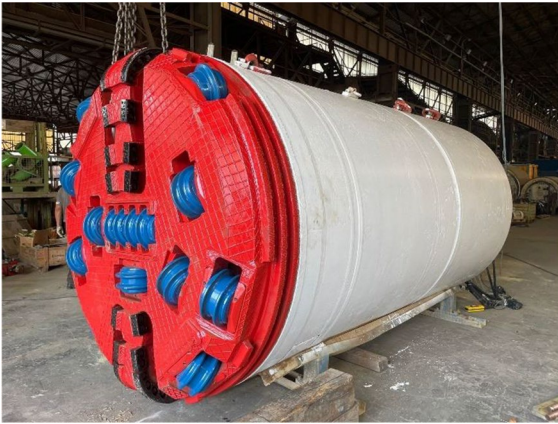
Fig. 1 Example of the micro-tunnel machine used for the construction of small diameter tunnels
