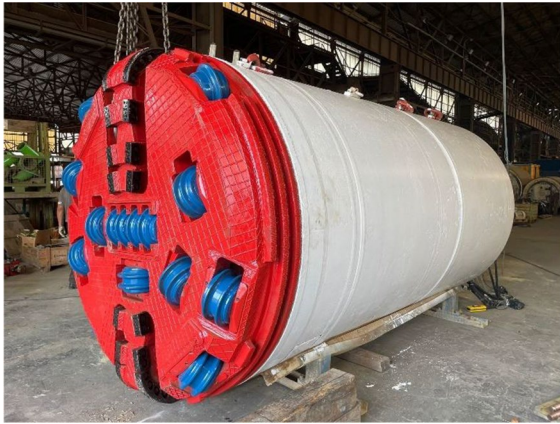
Fig. 1 Example of the micro-tunnel machine used for the construction of small diameter tunnels
