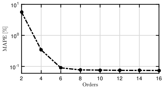
Figure 18: Approximation error (MAPE) between the target frequency response and the reduced order model frequency response, for different model approximation orders \nu .
