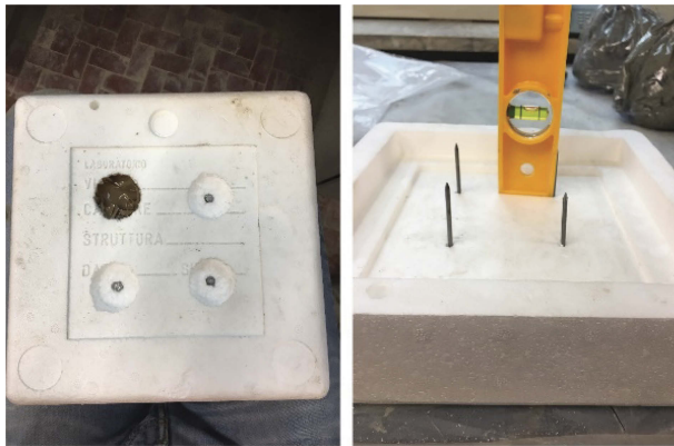
Figure 3. Polystyrene support used for the samples production.
