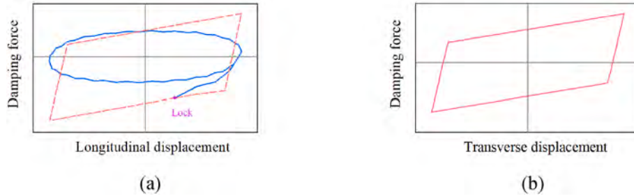
Fig. 2. The force-displacement relationship of HBHDS in the (a) longitudinal direction and (b) transverse direction.
