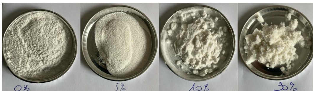
Figure 1: Macroscopic observation of particle size changes due to granulation (Avicel PH-101/Ethanol)
