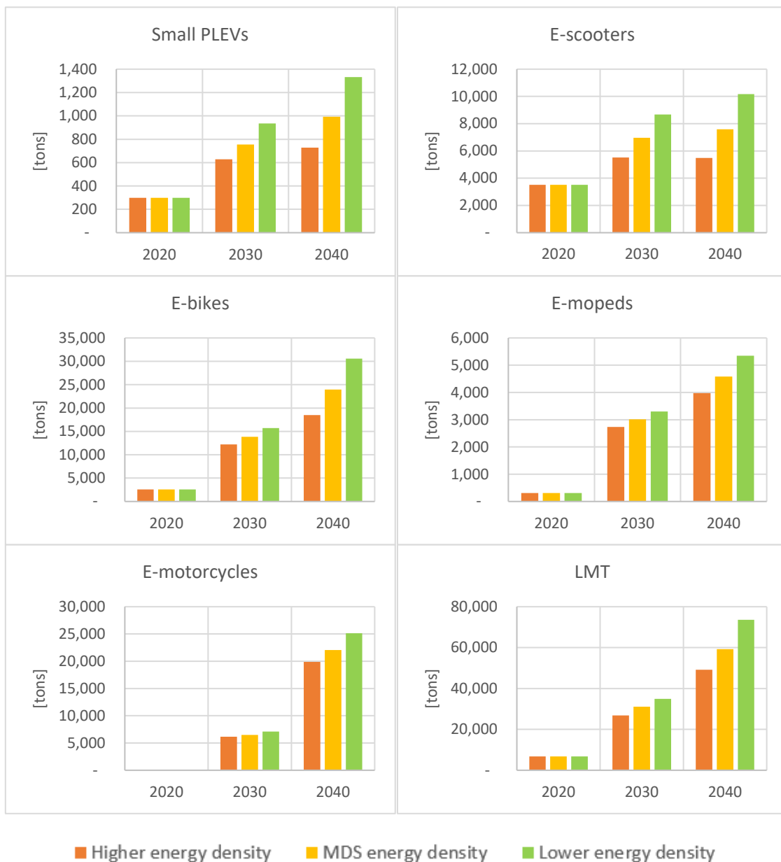
Figure 29: Tonnage waste batteries in 2020, 2030 and 2040 in Europe varying the energy density of batteries
