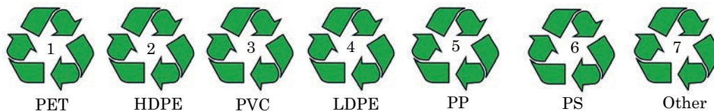
Figure 2.1 Plastic and recycling code according to ASTM D7611 / D7611M [3]
