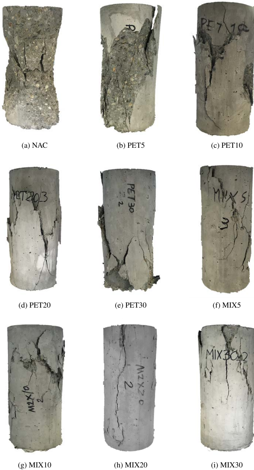
Figure 7.9 Typical failure modes under static loading of standard cylinder specimens for NAC, PET and MIX with different r.
