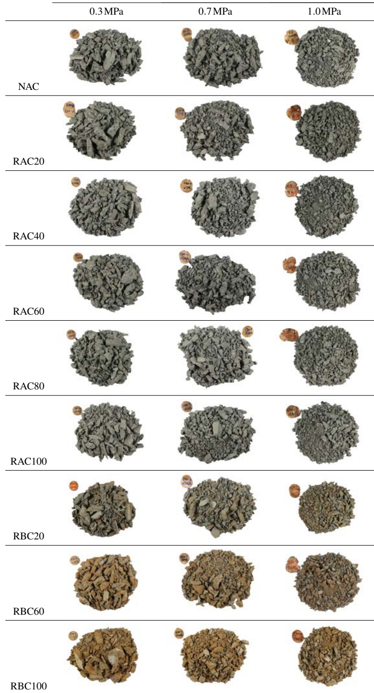
Figure 4.6 Typical failure modes of NAC, RAC and RBC specimens with different r after SHPB tests.
