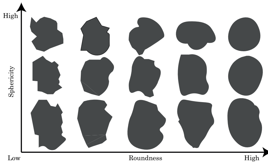
Figure 2.4 Classification and evaluation of particle shape (adapted from Ulusoy [4])
