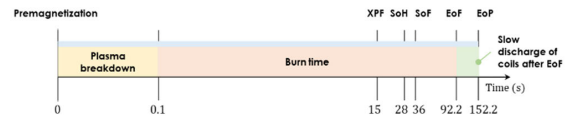
FIGURE 4. Timeline of the standard SN plasma operating scenario considered in the present analysis.
