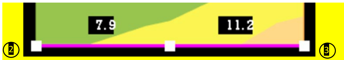
Fig. 4A. Section at the base of the wall depicted in the Dolmen, bounded by vertices 2 e 3, subjected to wind load acting along the X direction, with shear stresses in [daN/cm 2 ].
