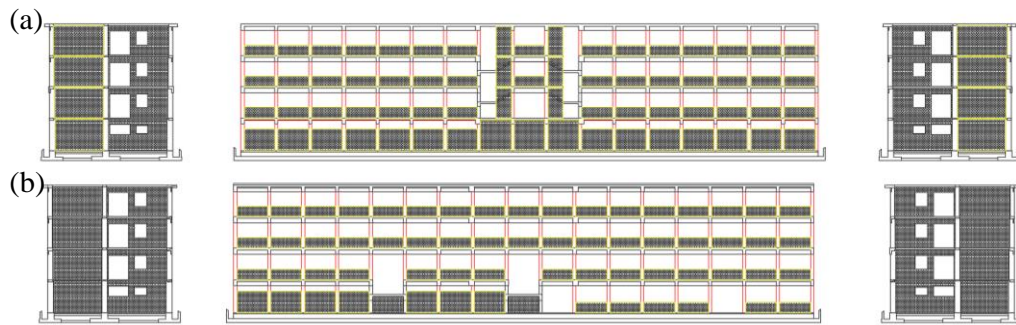
Figure 3: Actual disposition of the external infills in the RC frames.
