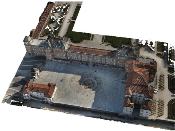
Figure 17. Photorealistic textured 3D model of the Reggia di Venaria. Mesh composed of 68'051'593 faces and 34'045'434 vertices.
