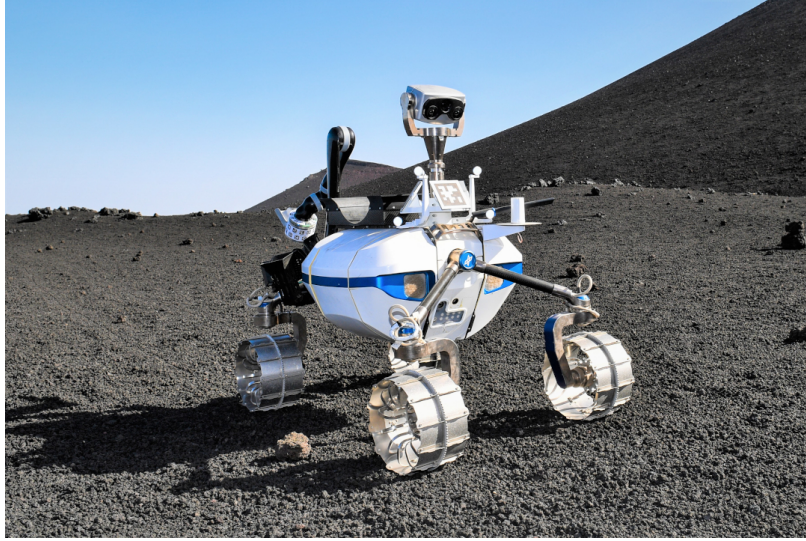
Figure 5: The Light Weight Rover Unit (LRU) including manipulator, docking interface and payload carrier.
