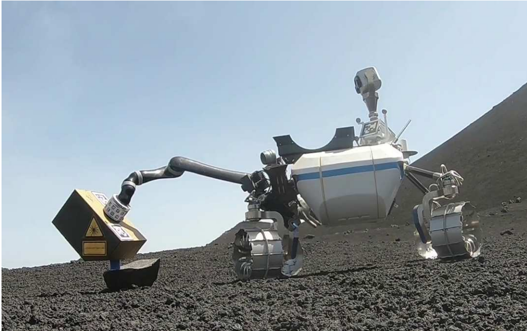
Figure 1: The Light Weight Rover Unit measuring a rock with the LIBS instrument at the analog test site on Mt. Etna.
