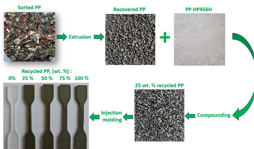
Figure 8. Reprocessing of recovered PP by compounding it with virgin material.
