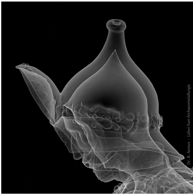
Figure 5. Based upon a 3D scan of Theoderich and the total weight of this statue, an average wall thickness was calculated. For visualisation purposes a hypothetical uniform layer was applied on the inside. 3D scans of the models would certainly aid in the interpretation of how the models were made (Foto: B. Asmus).
