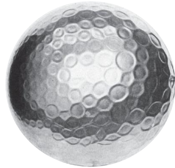
An electroplated nickel shell that has been continuously pressurised around a slightly smaller internal spherical mandrel [Carlson, et al 1967].
