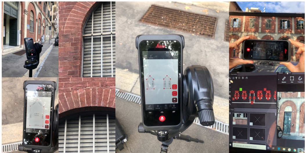
Fig. 07. BLK3D during point acquisition and image processing within the backoffice survey return platform. Image by author
