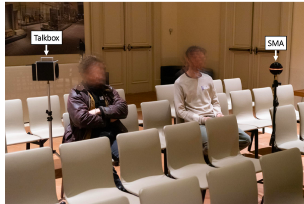
Figure 26: Picture of the RIR recording procedure in case of SMA placed in the farthest listening location (L2) and the Talkbox placed in the respective 120° azimuth noise location (N2120°).
