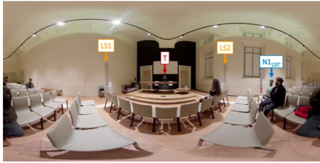
Figure 28; Equirectangular preview of the visual scene with the listener closer to the target speaker (T) represented by the Talkbox in the front and the one-talker noise at 120° azimuth (N120°) represented by the dummy-head.
