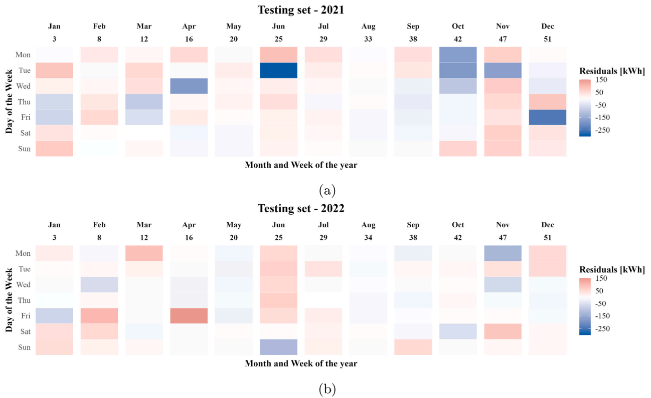
Fig. 8. Residuals between the estimated and actual daily electrical energy consumption values for 2021 (a) and 2022 (b) using the BART model.
