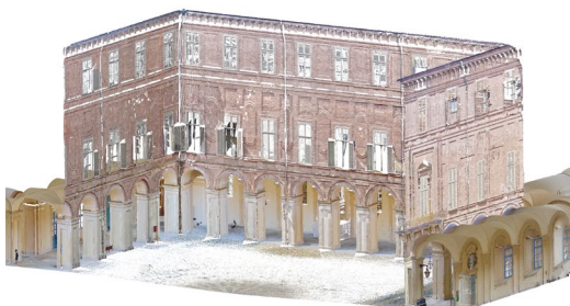
Figure 3. Flash point cloud of the Royal Palace's cloister.
