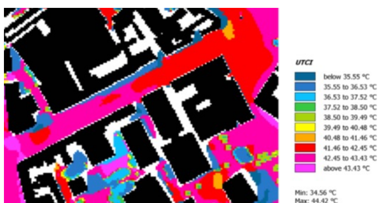
[Sch 1] Figure 12. UCTI Simulation of the Current Status at 16.00 pm of 21.06.2018. Source: Authors' Elaboration - ENVIMET Simulation
