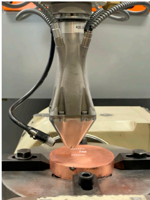
Figure 1. Prima Additive Laserdyne 795 with the REAL_DED ® coaxial deposition head featuring a laser spot of 2 mm in a 7 mm working distance.
