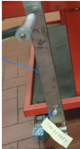
Figure 2.9: Dovetail dummy blade on free-free conditions, accelerator attached
