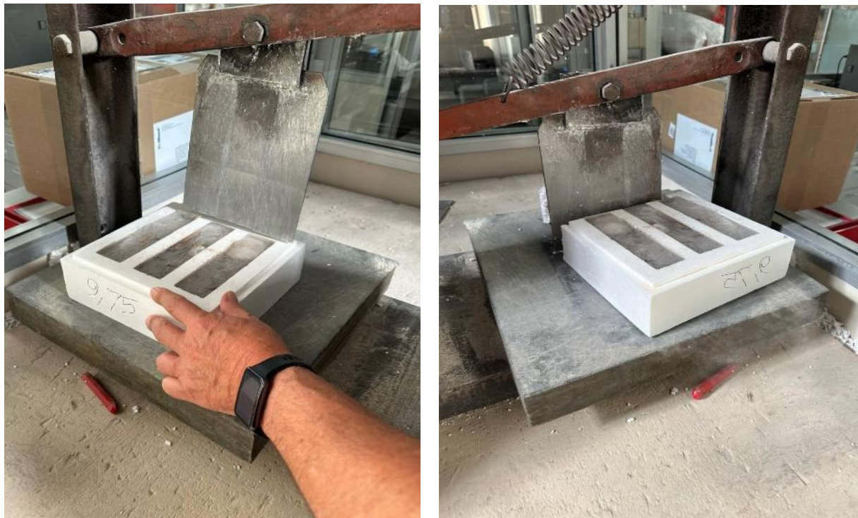
Figure 3.2: Polystyrene Molds for Ice Specimens.
