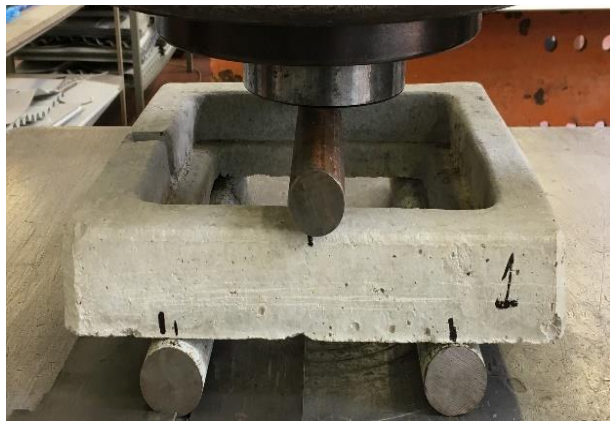
Figure 2.16: Three-point bending tests on concrete rings of manhole covers.
