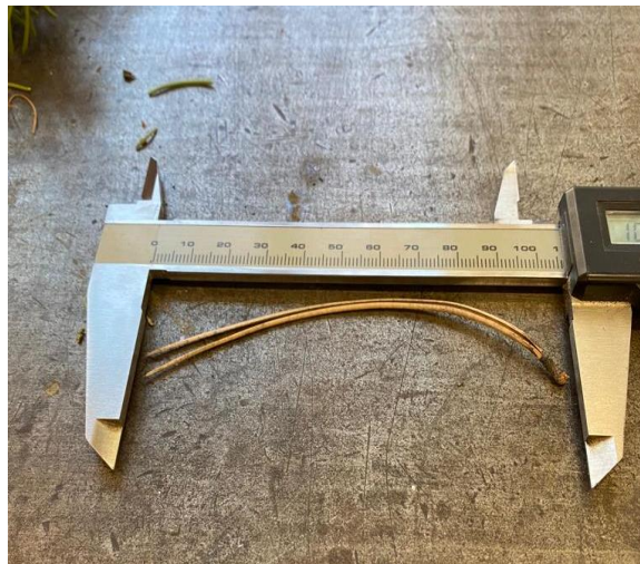
Figure 3.3: Pine needle used as fiber-reinforcement for ice.
