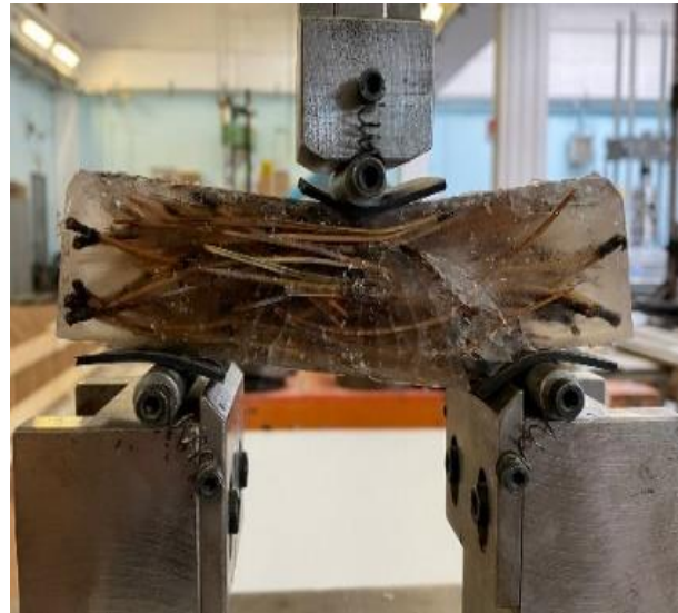
Figure 3.9: Results of three-point bending tests: (a) ideal P - \eta curve in the rising branch. (b) multiple cracking in the specimen.
