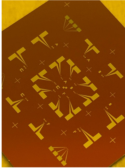
Fig. 3.1 Central layout pattern of the chip mask. The TESs are placed equidistant from the chip center to minimize thickness gradients.
