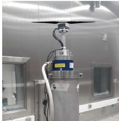
(a) Isolated T-Motor 15x5 rotor test in terraXcube
