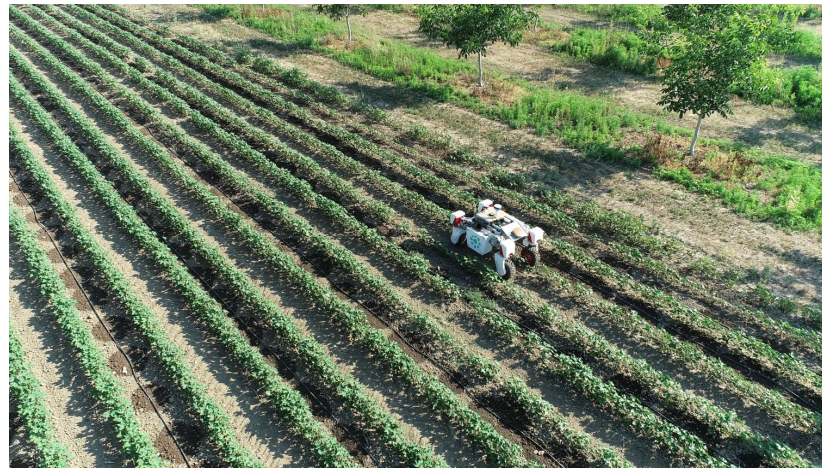
Figure 11. UGV following the adjusted tracks that were created in a cotton field.
