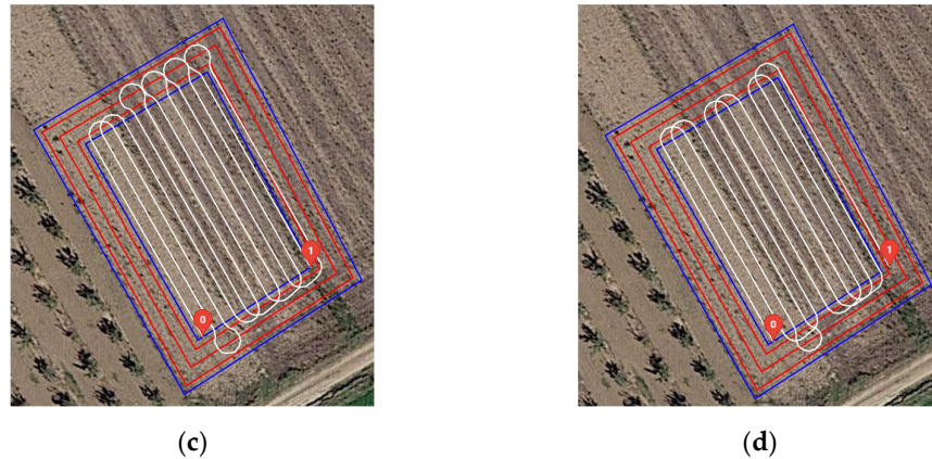
Figure 4. (a) AB pattern, (b) SF pattern, (c) BL pattern, and (d) an instance of B pattern. Numbers “0” and “1” refer to the starting and ending point of the route, respectively.
