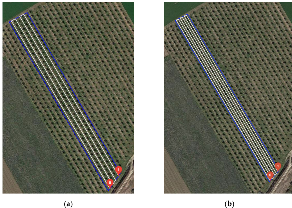
Figure 14. The fieldwork tracks of the experiment performed in a tree orchard. (a) Routes performed in the middle of the row; (b) routes dedicated to one side of the tree row.
