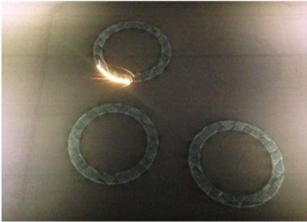
Figure 4: Exposing with contour parameter from Gradl et. Al., 2018 [1]
