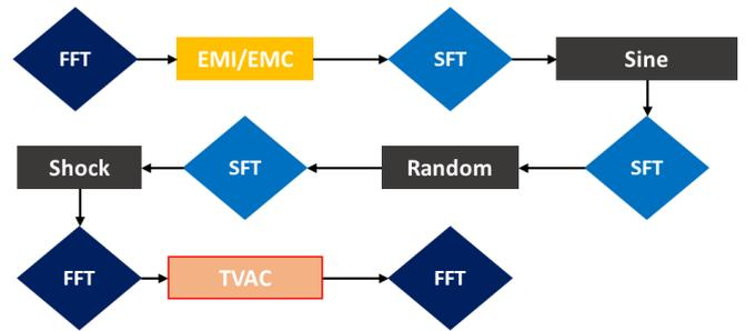
Figure 5: QN400-SPACE EQM Receiver Qualification Test Campaign
