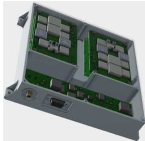
Figure 4: LuGRE QN400-SPACE GNSS Receiver
