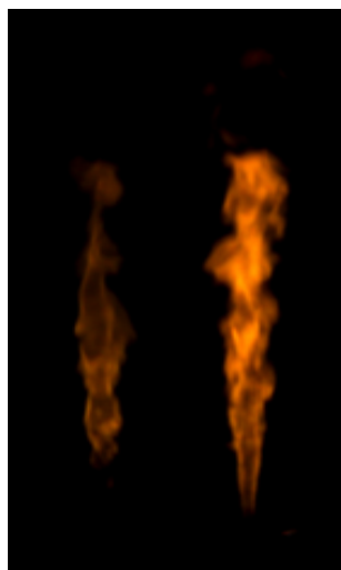
Figure 4.2.7: The ammonia/5%hydrogen jet flame at 973 K and 1173 K.
