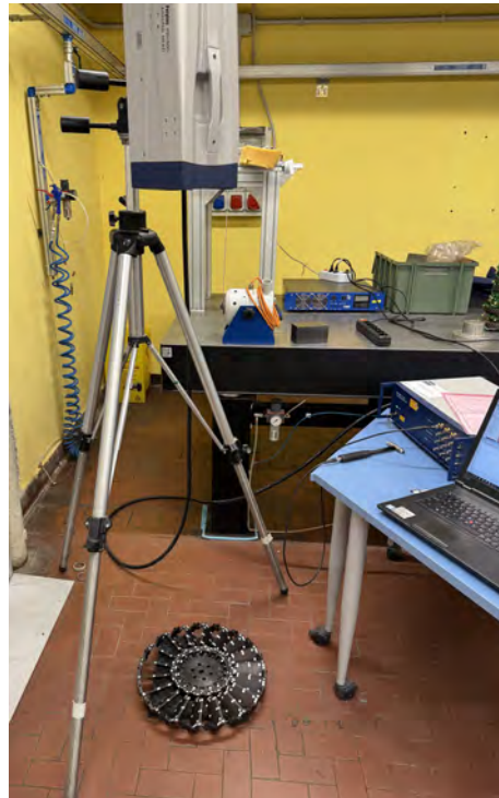
Figure 3. Experimental setup used for modal testing under free–free conditions, showing the LDV system, impact hammer, and data acquisition hardware.
