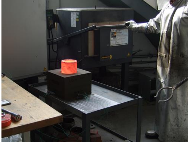
Figure 13: F-TPS finished sample during thermal test, [2].
