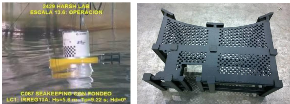
250 251 Figure 4 Experimental physical moored model subject to the sea state 10 as defined in Table 6, side view, (left) and bow landing upper view (right)
