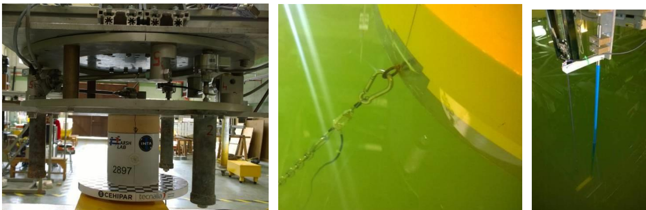
Figure 6 Six degree of freedom dynamometer (left) and load cells for line tension measurement (centre) and a wave elevation gauge (right)
