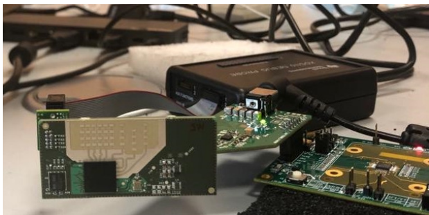
Fig. 10: Realized Radar board prototype
