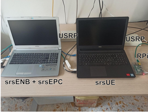
Fig. 10. The nodes of the lab test-bed we employ.
